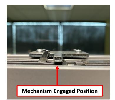
Test the mechanisms by opening and closing the door. In the correct position each trigger will pull the catch piece to engage the mechanism. When the mechanism contacts the trigger, the trigger will initiate the soft close and/or soft open function.
