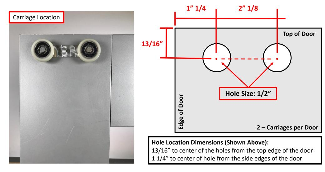
When installing Aluminum Framed Sliding Glass Doors the holes for the carriages will need to be pre-drilled, use the dimensions shown above for the hole locations. When drilling the holes only one side of the door will be drilled through, see next page for reference. We recommend drilling smaller pilot holes prior to drilling the 1/2" holes for the carriages.
