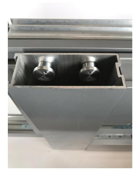
1. Install the Carriages into the C-Rail by pressing them into place or sliding them in from one end. Carriages to have the flat side down.
